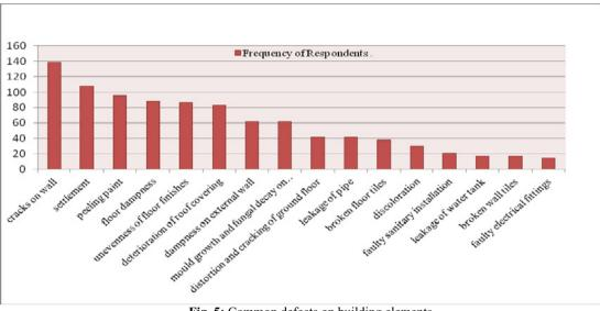
Fig. 5: Common defects on building elements
