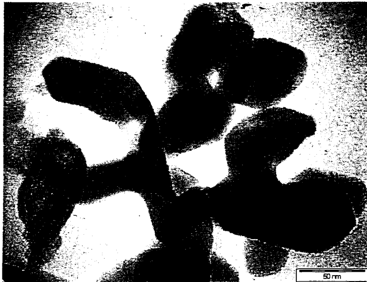
Figure 4.8: An EFTEM image of the nanostructures formed on a silicon wafer at the oxidation time of 2 min.
