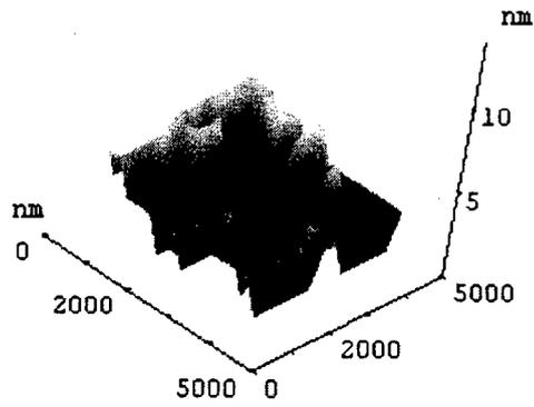
Fig. 3 Atomic force microscopy image of the Ni Schottky contact on the MSM photodiode under *A+C* treatment at 400°C.
