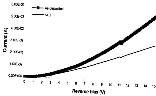
Fig.1 Current-voltage (I-V) characteristics of the samples annealed at 700°C
