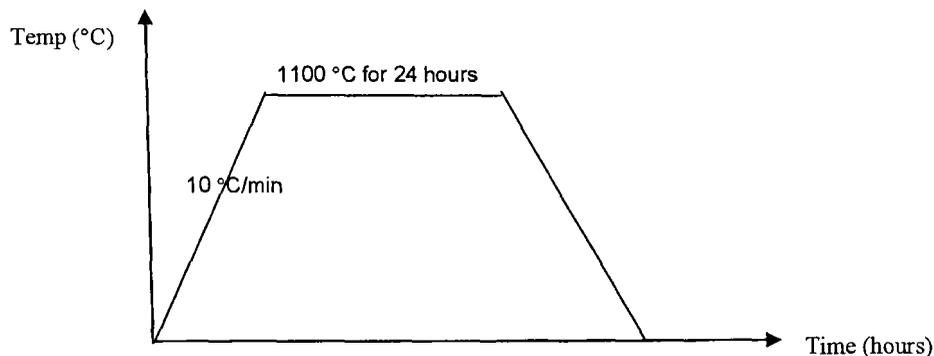
Fig. 2. Schematically temperature-time path used of the heat treatment process.
