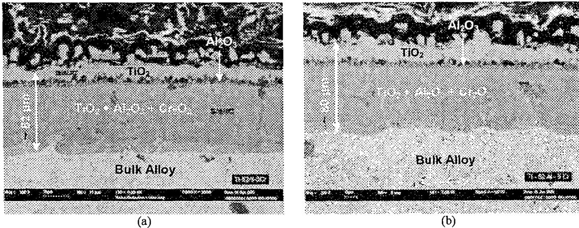
Fig. 9. Cross-sectional microstructures after oxidation in air at 900 °C for 50 hours of Ti-52Al-5Cr alloy with magnification 500x (a) before heat treatment; and (b) after heat treatment.
