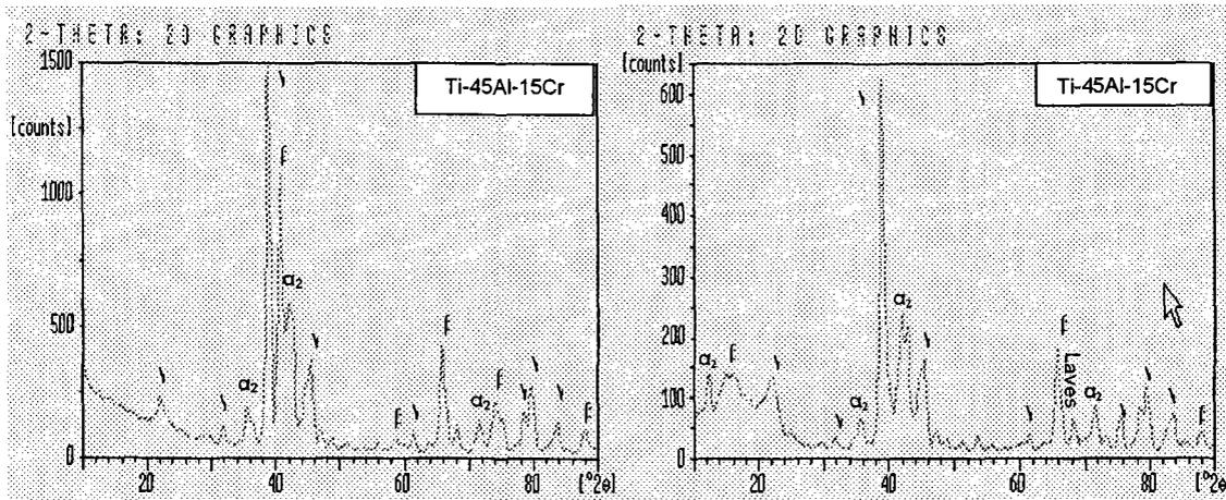
Fig. 8. X-ray diffraction patterns of Ti-45Al-15Cr alloy (a) as-cast alloy (b) heat-treated alloy.
