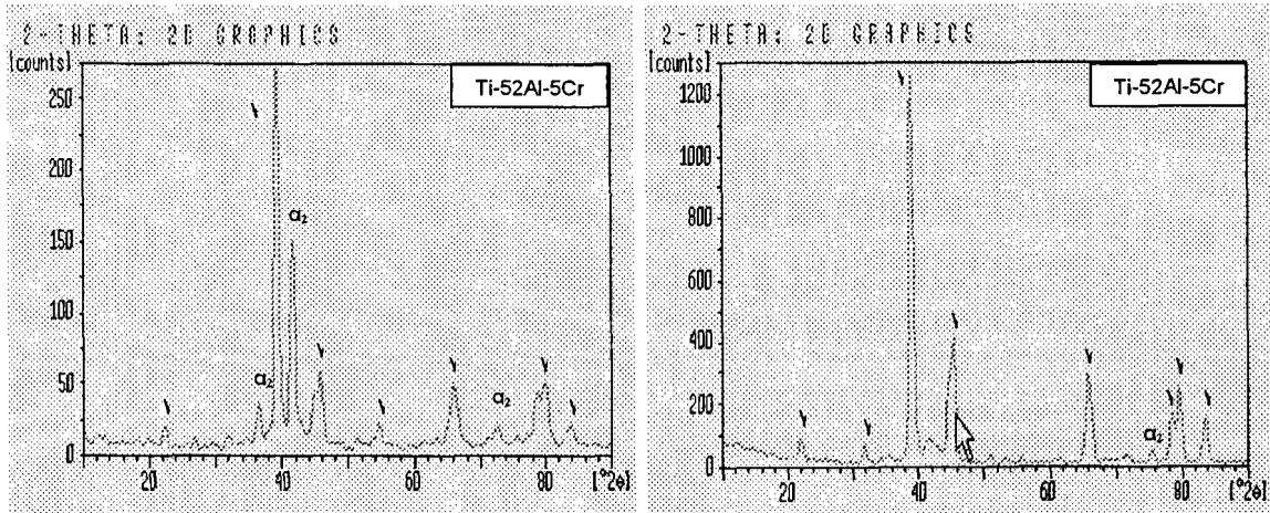
Fig. 6. X-ray diffraction patterns of Ti-52Al-5Cr alloy (a) as-cast alloy; and (b) heat-treated alloy.
