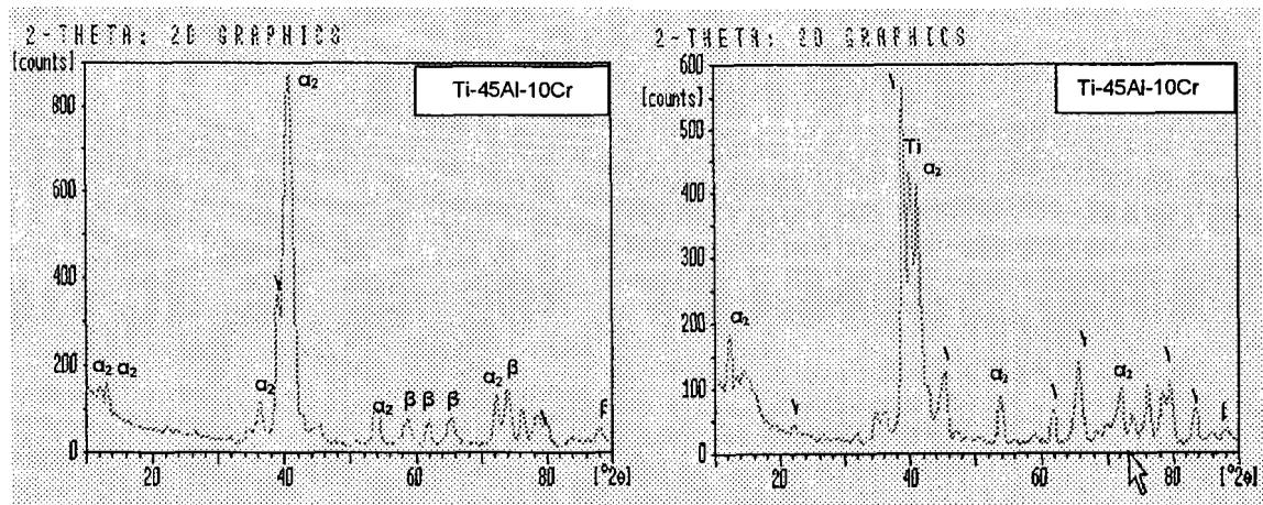
Fig. 7. X-ray diffraction patterns of Ti-45Al-10Cr alloy (a) as-cast alloy; and (b) heat-treated alloy.
