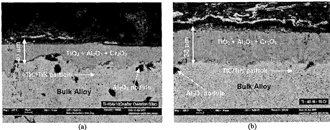
Fig. 10. Cross-sectional microstructures after oxidation in air at 900 °C for 50 hours of Ti-45Al-10Cr alloy (a) before heat treatment (with Mg. 250x); and (b) after heat treatment (with Mg. 500x).
